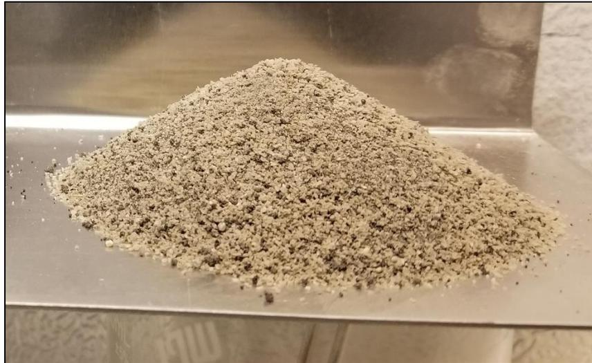
**Figure 5.2.2.** Granular Icy Regolith Simulant, 12% Water Weight.
