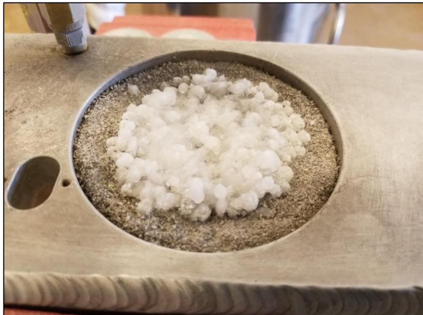
**Figure 5.2.5.** Frost Layer Production, Simulant and Container at 77K.
