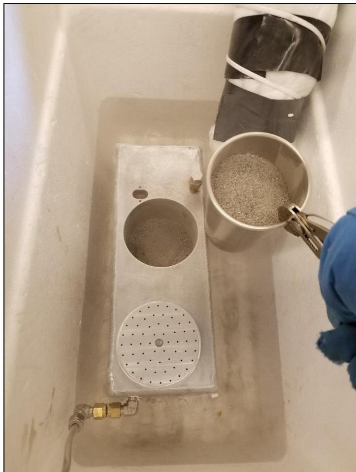
**Figure 5.2.3.** Block 1 sample container submerged in LN with LN feed through.
