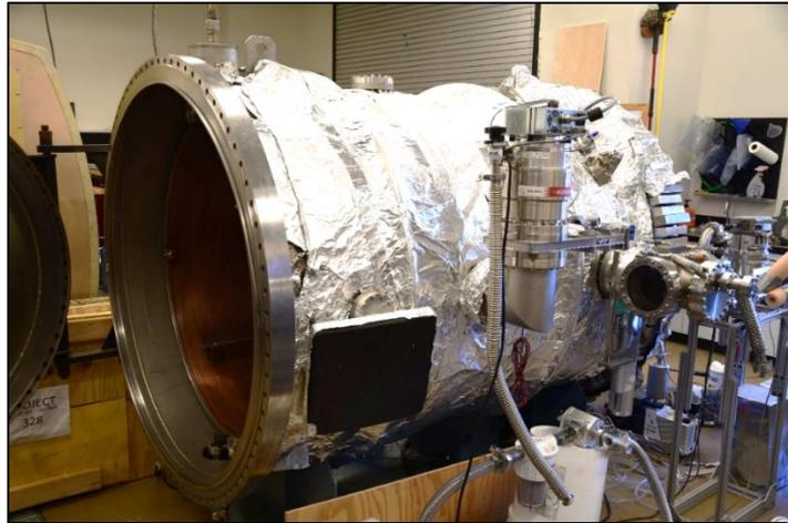
**Figure 6.2.** The large (2.7 m<sup>3</sup>) cryogenic vacuum chamber at CSM.
