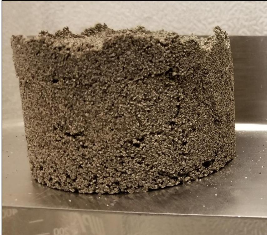
**Figure 5.2.4.** ‘Mud pie’ icy regolith simulant, 12% water weight.
