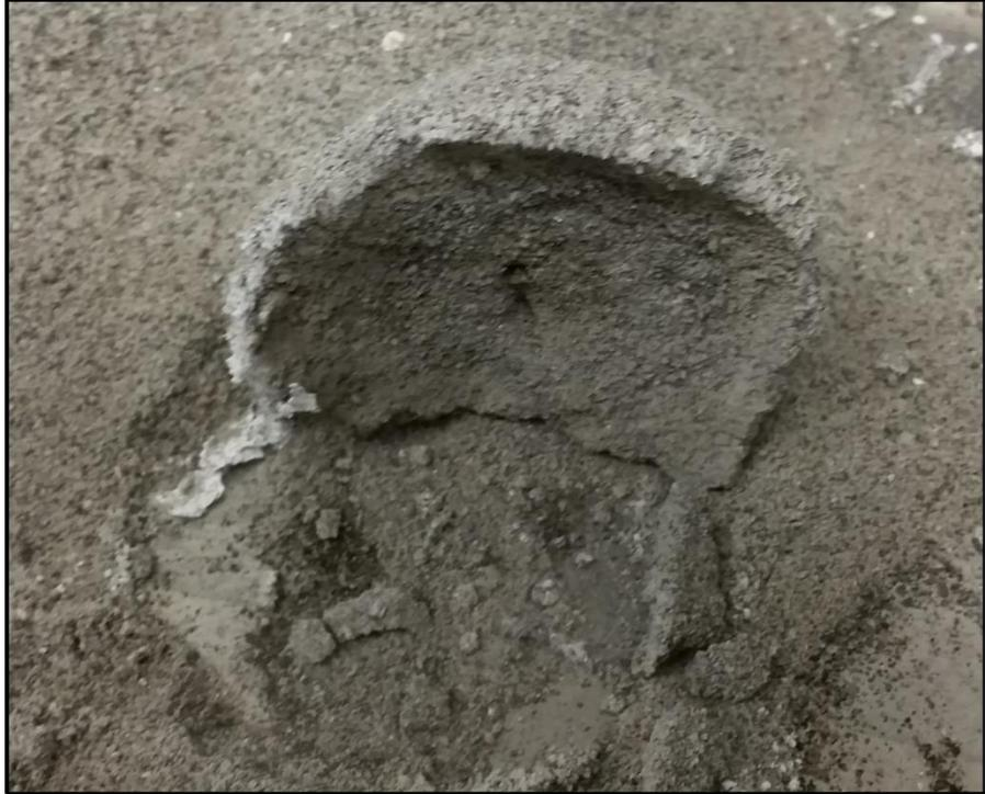
**Figure 5.5.3.** Typical lens found in 5.6% and 12.0% granular tests.
