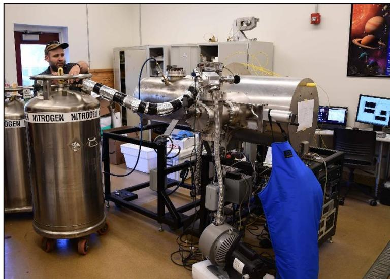
**Figure 1.4.** CSM medium cryo-vacuum chamber.
