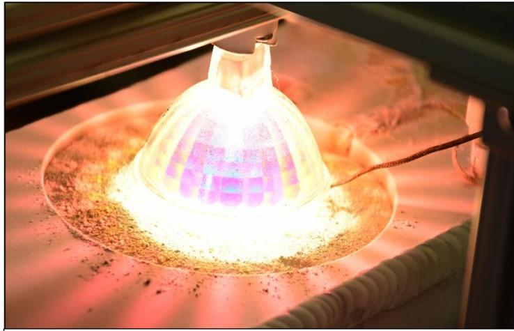
**Figure 2.2.** Heat applied to an icy regolith simulant sample under cryogenic vacuum conditions.
