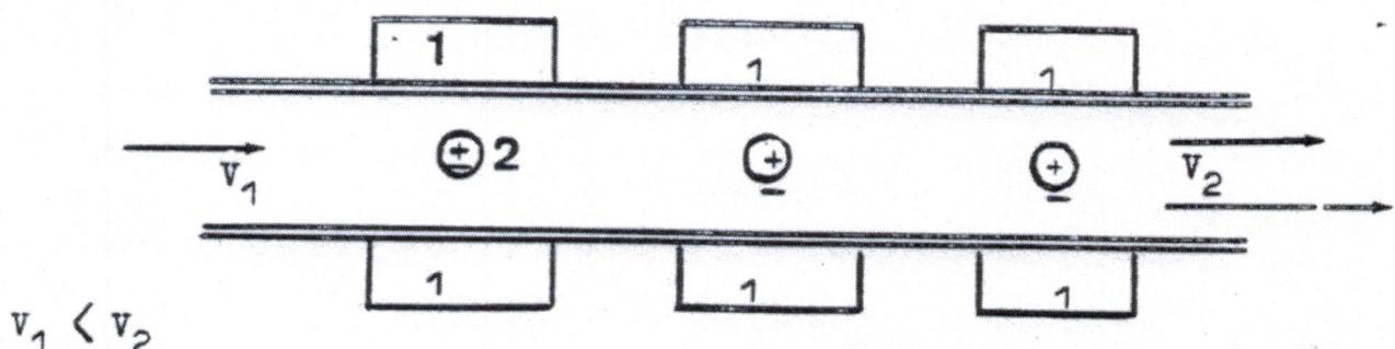
3 Magnetogasdodynamic (as motor for materials movement) before introduction in PLASMA CHAMBER 4 ( microdivision plasma chamber ).
